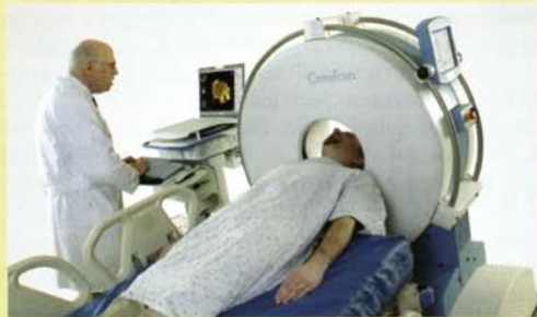
Neurologica's portable CT scanner can be wheeled to the patient bedside to scan the brain. The CereTom system, released commercially about one year ago, is used primarily in the ICU and ER. (Provided by Neurologica)
