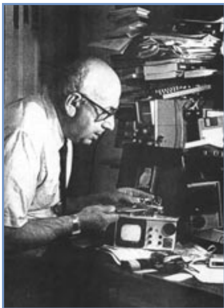
Morris Soled, MD, working on the battery-run oscilloscope that he designed, built and used for house calls.
